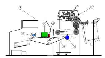
Figure 3. Combination of offset press and inkjet imprinting unit. 1: Quickmaster 46-1 offset press, 2: inkjet imprinting unit, 3: vacuum cylinder, 4:vacuum belt, 5:paper edge sensor, 6: inkjet heads, 7: UV dryer
