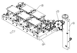
Figure 2. SP12.8/600 Single Pass Print Engine. 1: Last chance filter; 2:Five 2.56 inch print swaths; 3:Frame; 4: J-tube
